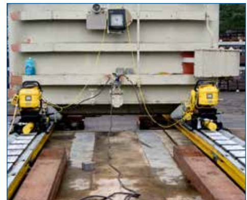
▼ A custom hydraulic Low-Height Skidding System for transport outage maintenance. Shown with optional track support. Both power units are connected together to provide synchronous travel of the load.
