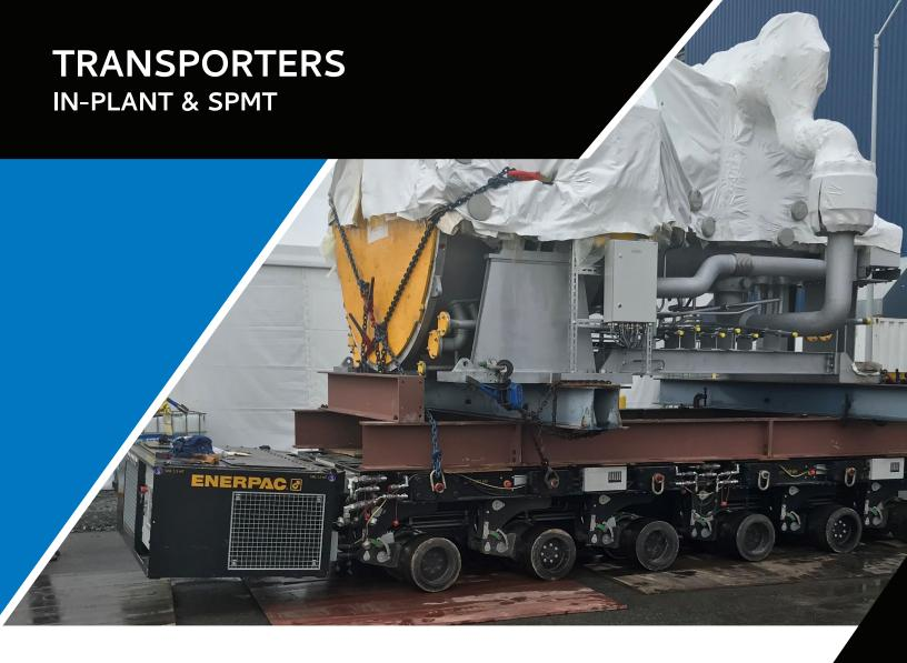
Our In-Plant Transporters and Self-Propelled Modular Transporters (SPMTs) provide a game-changing ability to move heavy equipment through small entries and tight corridors. The pivoting wheel assemblies allow the trailer to move forward, backward and sideways. With a self-sufficient power source that eliminates power cords, the unit can rotate 360 degrees without changing its midpoint. It fits where other trailers can't!
