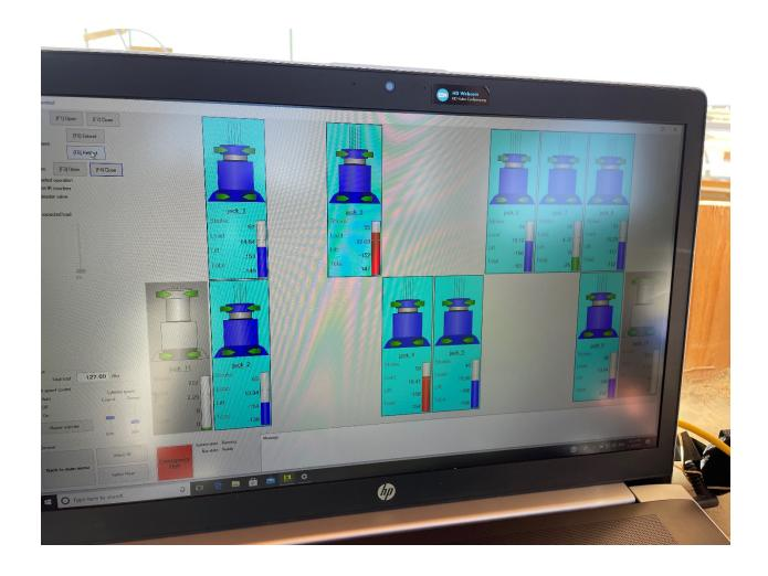
"We could see how the individual strand jacks were responding, and we tuned the system to automatically accommodate the imbalance," Cox added (see photo above). "We developed one set of parameters that accommodated about 80 percent of lifts and several other custom configurations for the outliers."
