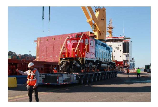
railroad tracks. Using the gantry system, the team lowered the locomotive onto the tracks and repeated the maneuver two times. The three locomotives were unloaded and transported to the tracks in just nine hours.
